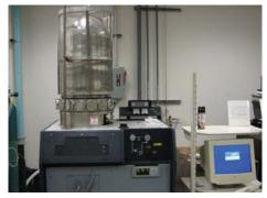
Thermal Evaporator Resistance evaporator for thin metal films
